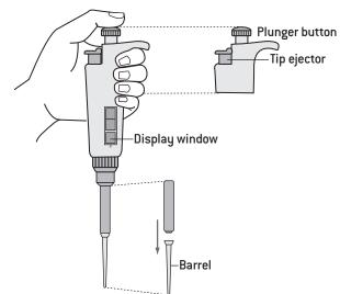
• When aspirating (drawing up) a solution, push the plunger to the *first stop* and lower the pipette tip below the level of the solution
